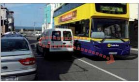
Figure 4.45: Setback stop lines allow for additional vehicular manoeuvrability for larger vehicles at signalised junctions without the need for larger corner radii.
