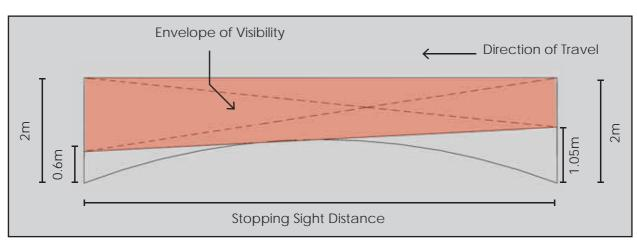
Figure 4.67: Visibility envelope in vertical plane.
