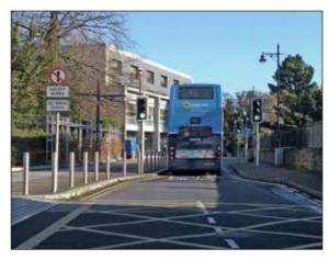
Figure 3.29: Example of a 'bus gate' in Tallaght, Co. Dublin, which filters permeability to allow for the free passage of buses whilst excluding other vehicles.
