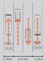
Standard lane/carriageway widths for multi lane *Arterial* and *Link* streets, including bus lanes. Range for low to moderate design speeds.
