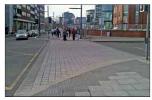
Figure 4.58: Examples from Tallaght, Co. Dublin of a robust surface material (including a slight vertical deflection) designed to add value to place and increase pedestrian safety by alerting/slowing vehicles on approach to the crossing.
