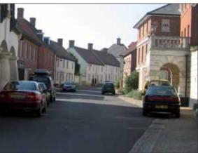
Figure 4.70: Examples from Poundbury, Dorchester, UK, where changes in the kerb line and carriageway alignment calm traffic by limiting forward visibility, creating pinch points and requiring multiple changes in direction.
