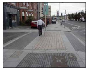
Figure 4.69: Example from Dorset Street, Dublin, where the carriageway has been raised and paved to slow turning vehicles and enhance the pedestrian crossing.
