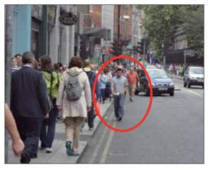
Figure 2.9: Footpath widths are inadequate, forcing pedestrians on to the carriageway, however, the width of the vehicular lane is in excess of what is generally required.
