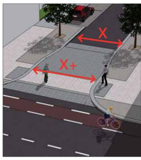
Figure 4.44: Illustration of how tighter corner radii can be applied to a junction, with additional manoeuvrability for larger vehicles provided by widening the street entrance.
