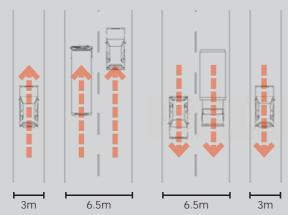
Carriageway widths for heavily-trafficked *Arterial* and *Link* streets in boulevard configuration. Main carriageway suitable for moderate design speeds. Includes access lanes with a lower design speed.
