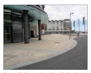
Figure 4.73: Example from Clongriffin Co. Dublin, where the footpath, kerb line and vehicular carriageway are at the same level. Whilst pedestrian and vehicular space are still clearly defined, a greater sense of shared space is still created.
