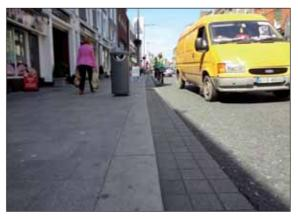
Figure 4.72: Example of a low kerb from Drogheda, Co. Louth, which is used to reinforce lower design speeds and create a greater sense of shared space.
