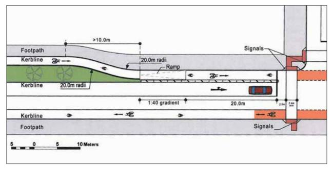
Figure 4.54: Extract from page 86 of the National Cycle Manual illustrating how to re-establish from an Off Road Cycle Track to Cycle Lane on approach to a junction. This design can be adapted to cater for onstreet parking by placing spaces within the green area or verge between the vehicular carriageway and Cycle Track.
