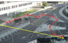
Figure 2.8: Examples of a junctions designed to minimise vehicle delays which significantly increase crossing times for pedestrians. Pedestrian desire lines (represented by the yellow line) are diverted through a series of separate crossings (represented by the red line). The top example can take pedestrians as long as 5 minutes to navigate.
