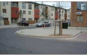
Figure 4.75. Example from Ballymun, Co. Dublin (top) and Leixlip, Co. Kildare (bottom) where kerb build-outs and contrasting materials are used to separate and define bays of parking from the vehicular carriageway, reduce corner radii and facilitate planting or landscape treatments.
