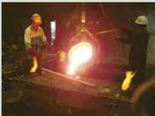
Pouring molten iron into a mould, Athy Co-Operative Foundry, County Kildare
