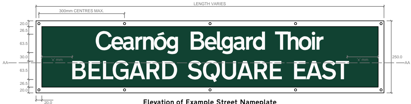
Elevation of Example Street Nameplate Scale 1:8
