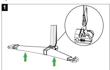
Align the spreader bar Quick-Connect latch at a 90 degree angle to hook. Insert the hook into the Quick-Connect.
