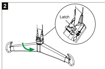
Move spreader bar to engage hook into the pivot. Rotate the spreader bar into position. Make sure that the Quick-Connect latch is closed.
