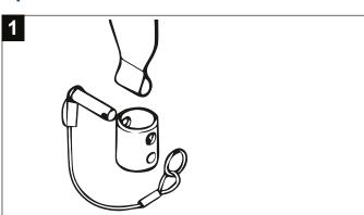
Insert the strap end onto the spreader bar attachment. Insert the clevis pin through the attachment and the loop at the end of the strap.
