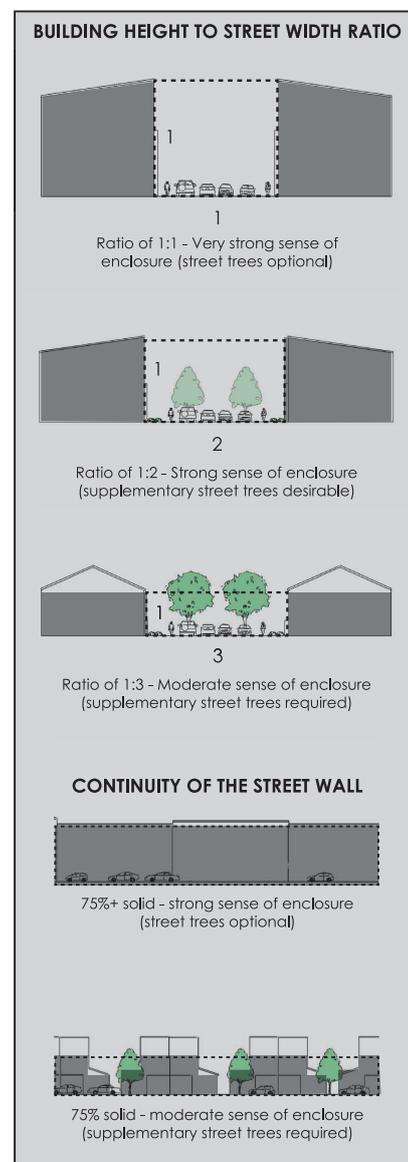
**Figure 3:** Building Height to Street Width Ratio - DMURS 2019.
