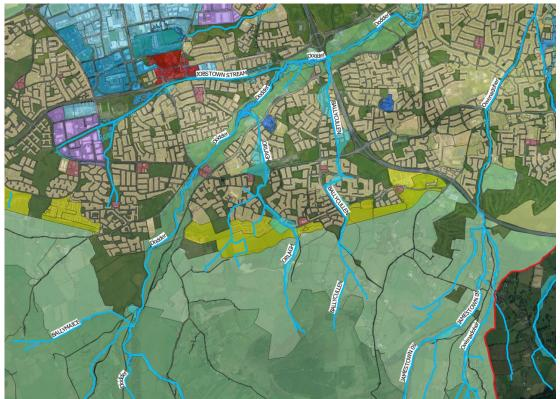
Figure 5.2 Ballycullen Oldcourt - Flooding extents over laid on zoning maps
